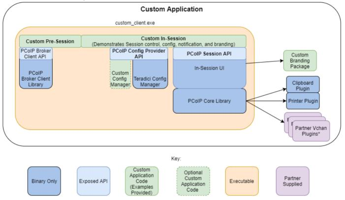
\*Partner Virtual Channel Plugins can be developed using the Virtual Channel SDK to enable this you can combine the PCoIP Client SDK with the PCoIP Virtual Channel SDK. For more information, see the Virtual Channel SDK.
